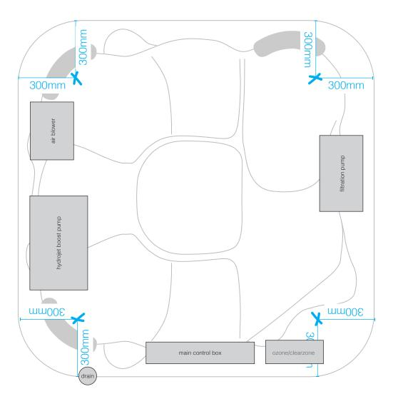
LOCATION FOR PRE-POWER THROUGH SLAB (power supply in conduit or flex to be installed in concrete slab at a MAXIMUM of 40mm above slab height)
